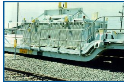
70-Ton Cask on rail car
