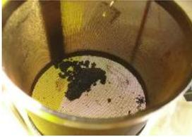
*Residual product after digestion of carbon matrix on unirradiated spheres*
