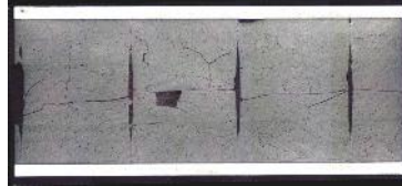
Pellet-Clad & Pellet-Pellet Bonding
